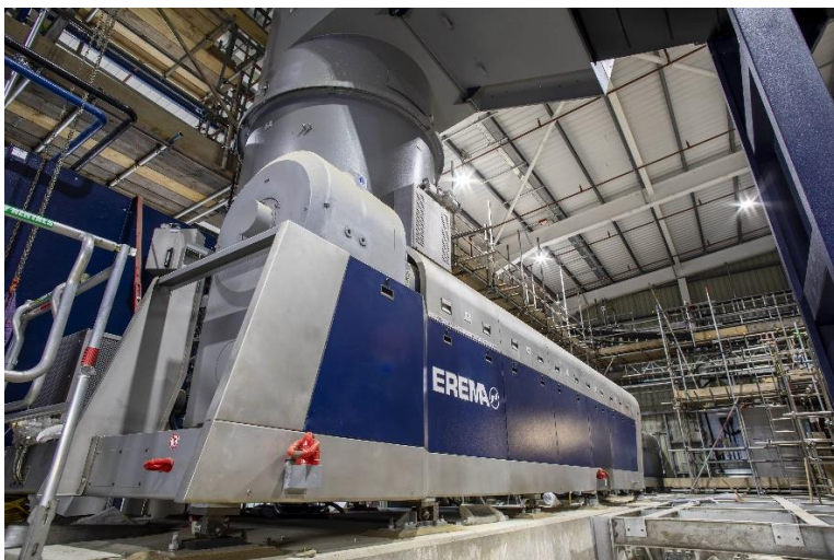
Caption: The EREMA CHEMAREMA® single-screw extrusion system for all input materials in chemical recycling
