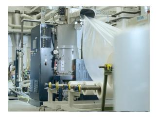
Fig. 2: The INTAREMA® K at Coveris is in operation 24/7. 100 per cent of the recycled material is put back into the film production process. Photo credits: EREMA
