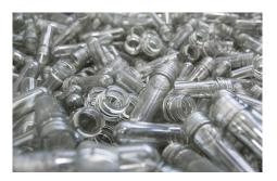
Picture 3: The PET Inline Preform system enables the flexible direct processing of PET flakes to make food contact compliant inline preforms in just one processing step.
