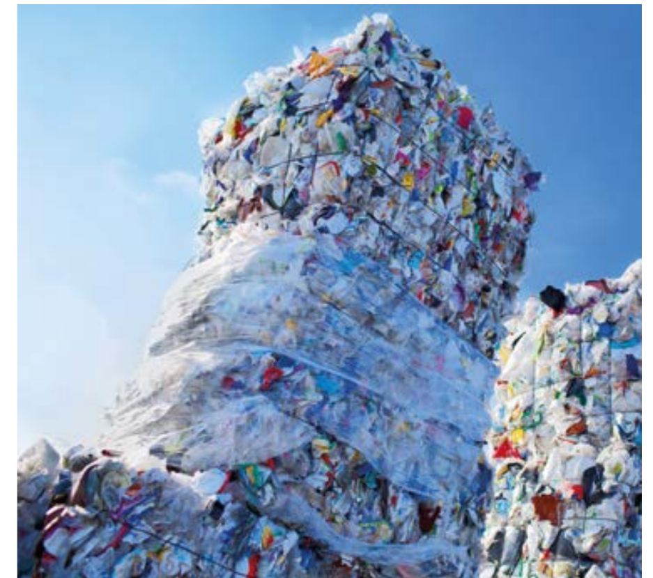
The raw material for the shower gel bottles is plastic waste sourced from what is known as the dual system, which is packaging material collected from households in Germany.
