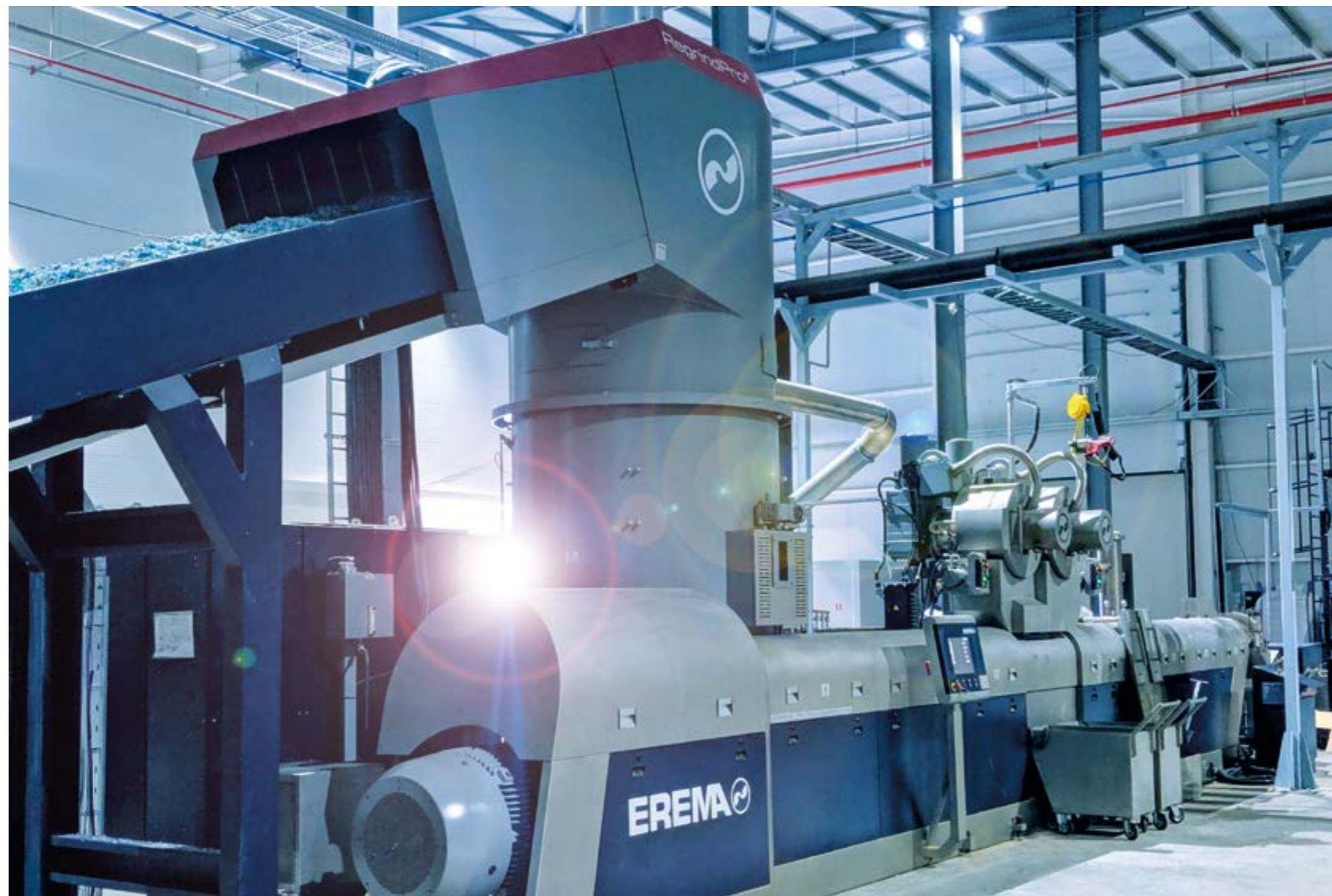
EREMA twin laser filter for efficient filtration: impurities such as paper labels, aluminium or foreign polymers originating from multilayer material such as PET or PA are reliably removed even at high levels of contamination of up to five percent.
