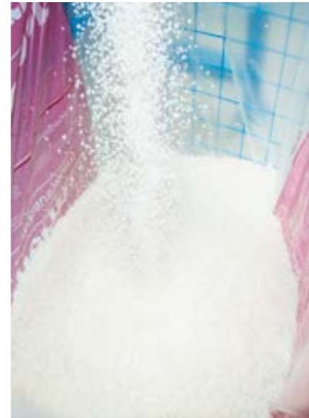
The finest quality flows into the collection sack: Coreth then processes the regranulate into high quality shrink and construction films; in the case of multi-layer films, it is used in the intermediate layer.
