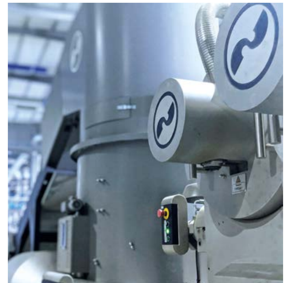
EREMA twin laser filter for efficient filtration: impurities such as paper labels, aluminium or foreign polymers originating from multilayer material such as PET or PA are reliably removed even at high levels of contamination of up to five percent.
