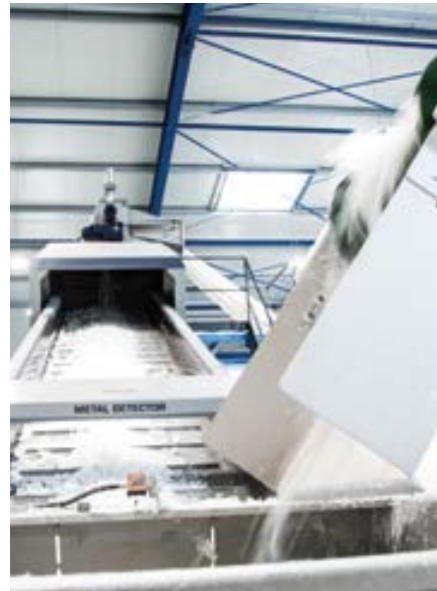
Lindner Antares and INTAREMA® TVEplus® in combination: The shredder transfers the shredded film flakes to the conveyor belt of the EREMA machine.
