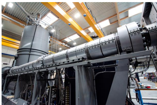
The reactor of the VACUREMA® T large-scale plant, which will go into operation in Brazil, almost reaches the roof of the new production hall, which was commissioned in 2021. From the Left: Patrick Rachinger, Product Group Manager, and Sophie Pachner, R&D Engineer. Photo: EREMA GmbH
