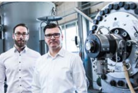
EREMA PET experts Michael Buchberger and Christoph Wöss in front of the VACUREMA® in the production hall at EREMA. The newly developed EREMA PET Laserfilter (right) processes input material with a degree of contamination of over one per cent without any difficulty and discharges the filtered particles continuously.
