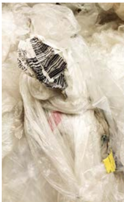
Plastics with impurities such as paper labels go directly into the recycling system.
