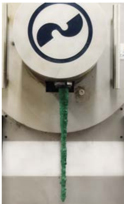
The EREMA Laserfilter has a continuous self-cleaning system which removes contaminants from the melt.
